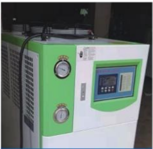
冷水机 COOLING WATER MACHINE
